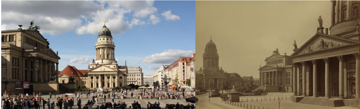
Figure 46: Difference between images taken during different time periods, which results in subideal texturing of the SfM reconstruction.
