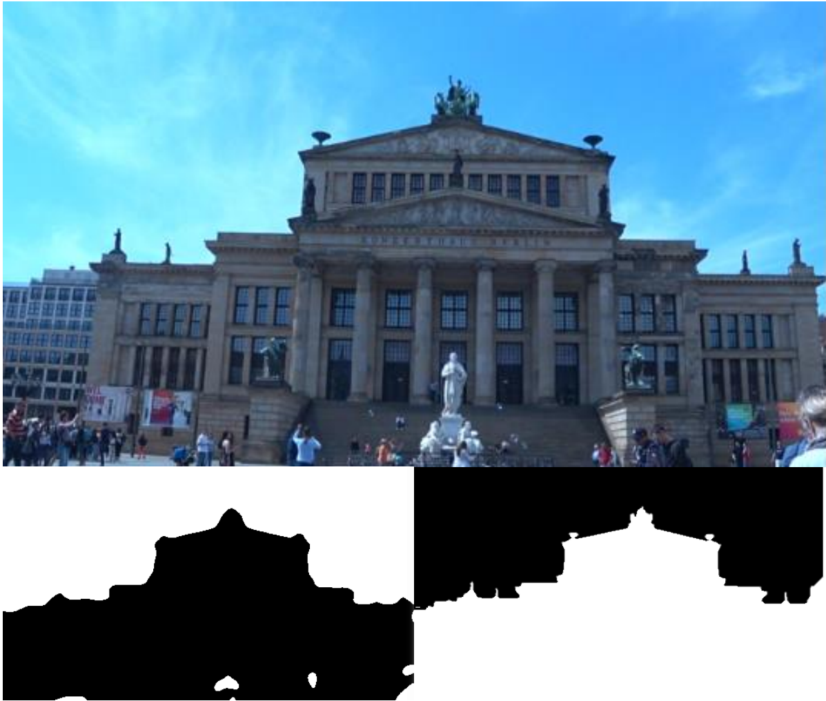
Figure 43: Masking results of the VGG16 CNN algorithm: (a) initial image, (b) building mask and (c) sky mask.
