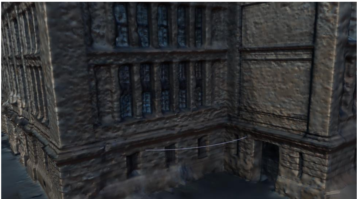
Figure 62: Resulting texture using all aligned input imagery showing blurred colours.
