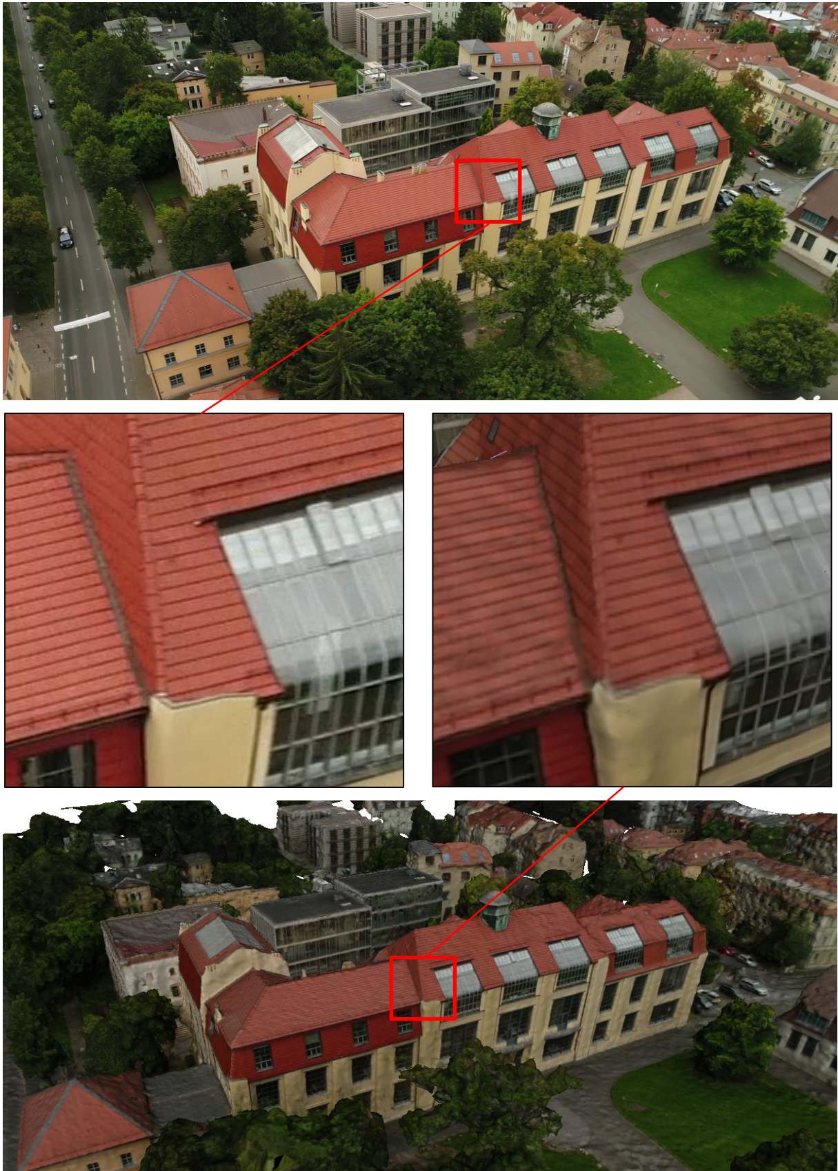
Figure 59: Texturing results Bauhaus universität: (top) image from drone, (left) zoom in of same image, (bottom) textured mesh and (right) call out of textured mesh
